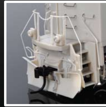
MU HOSES, COUPLER LIFT BARS AND TRAIN LINE AIR HOSES
